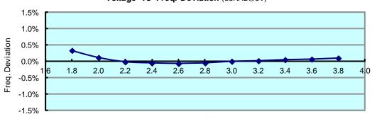
Voltage vs Freq. Deviation (38KHz@3V)
